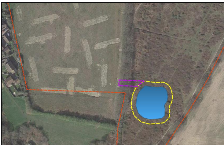
Figure 3: Area that would likely be impacted to allow for construction of the basin. Working room is identified in yellow and access route in purple.
