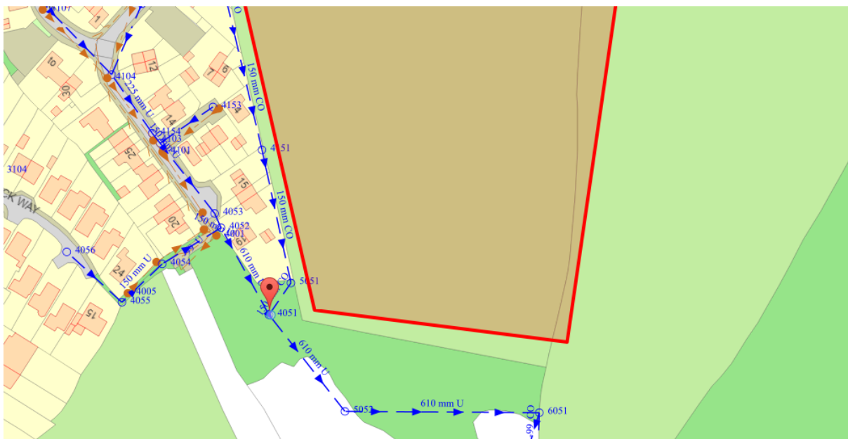
Figure 2: Surface water point of connection
