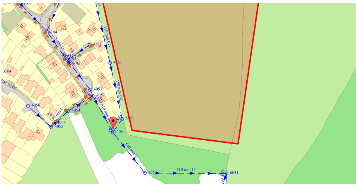
Figure 2: Surface water point of connection
